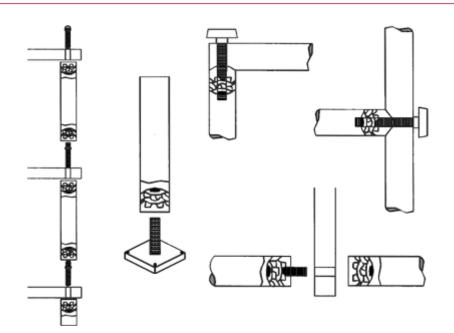
Inside Tube Diameter = 22,7-24,0 Outer tube diameter = 1" Thread = M6
